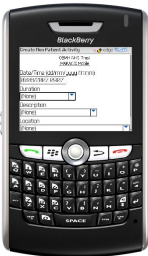
Non patient activity screen, only the input fields are 'active', date/time is entered using numeric keys (secondary use accessed by ALT key)
